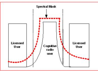
Fig.1.Spectral mask applied to CR user existing with licensed users
