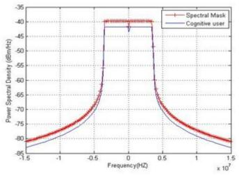
Fig.7 Proposed spectral mask without using notch frequencies
