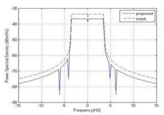
Fig.4. Spectral precoding using notch frequency technique
