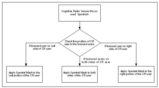
Fig.3.Efficient utilization of spectral mask techniques
